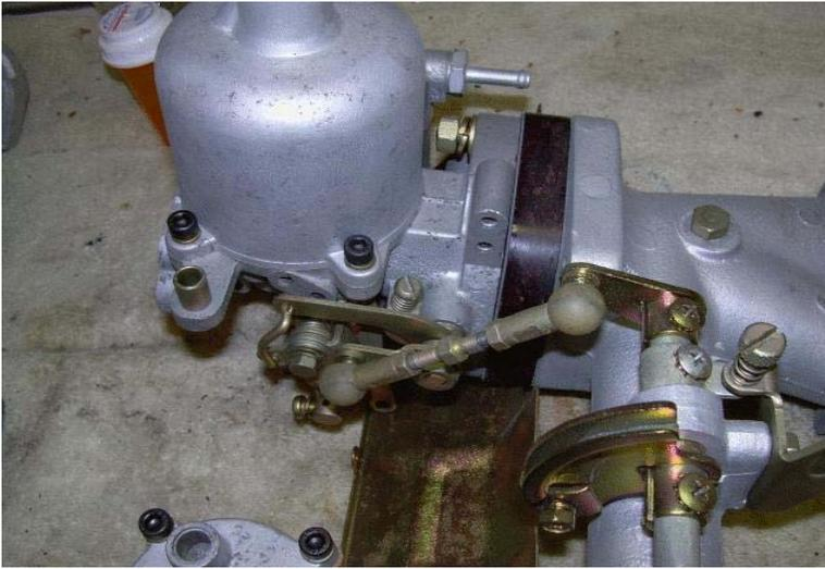
The "dog bones" are turnbuckles. It is not necessary to remove them to change the length. Loosen both lock nuts and turn the center section to vary the length. After the initial setup is done pick one dogbone to make future adjustments. This prevents them from getting progressively longer or shorter as you switch back and forth. I normally adjust the one closest to the firewall.
